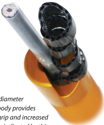
The MRT blade is spring-loaded and can be easily released. This enables the tool to slide without damaging the web and facilitates removal of a precise length of messenger.
