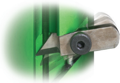
The MRT blade is spring-loaded and can be easily released. This enables the tool to slide without damaging the web and facilitates removal of a precise length of messenger.
